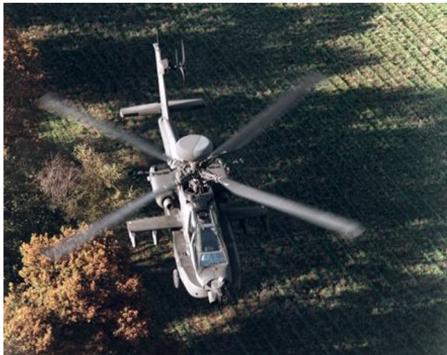
British army Apache Longbow, the radar can be seen on top of the main rotor mast. Photo: Rolls-Royce
